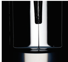
Fig. Tubeless siphoning of polyethylene oxide (PEO) solution
