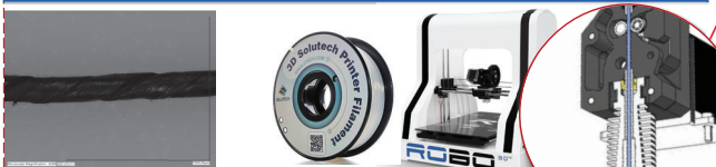
As-spun CNT yarns and 1.85 mm. diameter commercial PLA filament is fabricated by ROBO 3D™ R1 plus FDM printer
